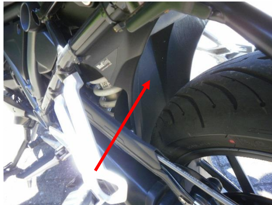
Rear suspension protector – without it, the suspension is fully exposed to the weather
