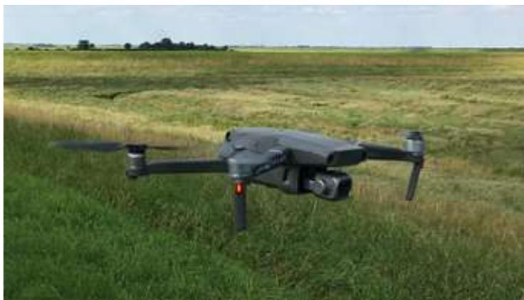
This whole kit was described to us as being 'mid-range' costing a mere £2600! From memory, it could climb to about 400 feet, with a range of 3 to 4 miles and can fly at 50 mph. Twin joystick operation was remarkably easy to control as he let me have a go.
